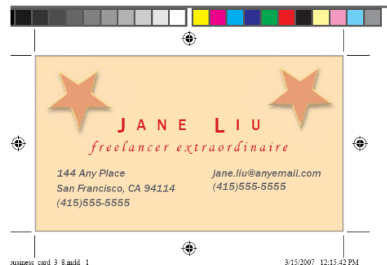
Figure 5 Printed file with printer's marks
