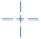
Used to locate the center point of holes or the central axis of a cylinder
